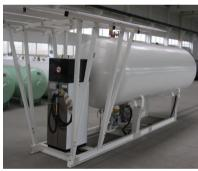
Pump protection *Differpress* protects the Red Jacket pump against the dry running, continuously measures and displays the pressure in the pipeline behind the pump.
