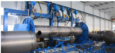
Our tanks are manufactured on new and modern machinery (welding machines from Germany, rollers from Switzerland). Thus we achieve manufacturing quality and productivity.
