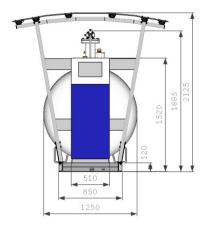
Autogas filling skid with submersible pump Red Jacket/Ebsray without shaft, with dispenser of any manufacturer, is the cheapest option of the unit. The pump is placed directly in the tank, and for the pump servicing the tank must be emptied.
